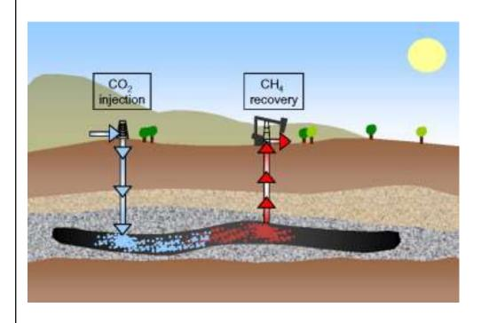
"Captured CO<sub>2</sub> is used to displace the adsorbed methane molecules and increase methane production"
